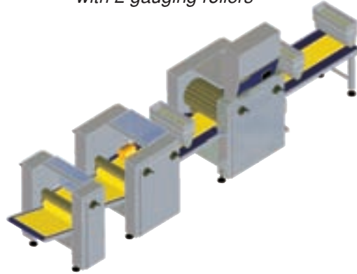
Dough billets laminating line with 2 gauging rollers
