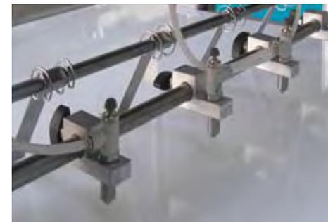
The humidifier is easy to adjust, to moist the portion of dough you choose. It's made with st/st upper tank, with gravity system, drop deposit and spreading unit.
