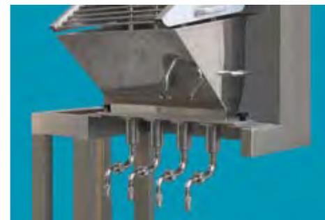
Supported by a strong, independent st/st structure, it is suitable for liquid fillings with small inclusions.
