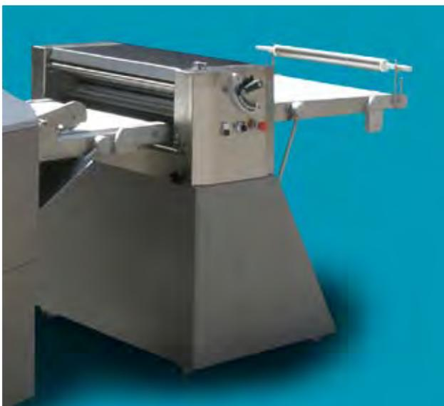
Installed at the entrance of the table, it grants an even thickness of the dough for precise processing, constant weight, etc.
