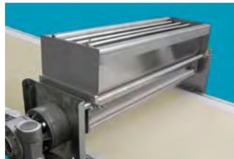
It's a roller device, it grants an even, adjustable, sprinkling of flour or sugar. The st/st hopper is easy to remove and easy to clean.
