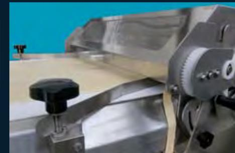
They remove and collect lateral scraps; scraps are collected in containers to be recycled.
