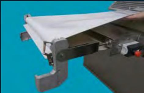
A quick releasing device for belt tension allows easy and careful cleaning of the table.
