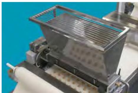
Interchangeable heads. Roller head to deposit hard dough; pump head for liquid fillings.
