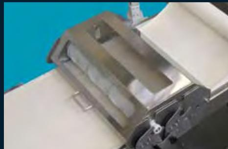
The table is pre-set for the installation of 2 rotating cutting dies, with total safety protection, to cut/mark/decorate the dough.
