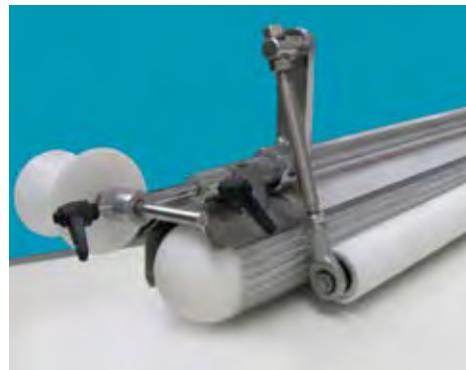
Made of a rolling unit and a counter-pressing roller, to automatically roll the dough (already filled) for cinnamon rolls.
