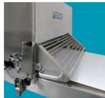
Different safety devices can be installed, in order to contain the size of the guillotine.
